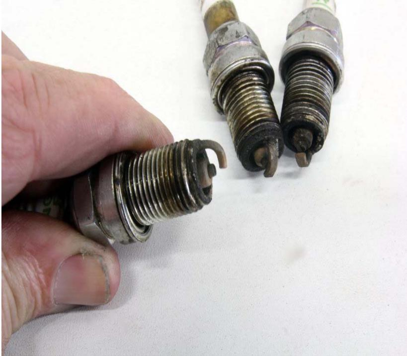
**This is a used plug from a small-block Chevy that had started out with roughly 0.040-inch gap and the copper core has worn to 0.050-inch. A wider gap increases the load on the ignition system, demanding higher voltage. Replacing this with a fine-wire plug would allow running a decent plug gap and still offer the potential for improved combustion.**
