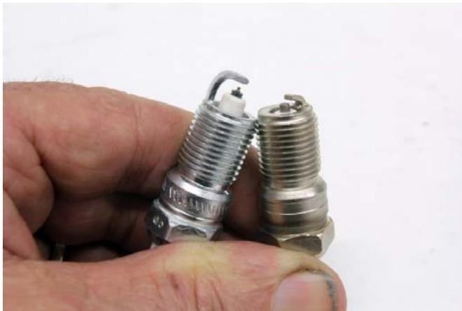
**Fine-wire plugs like this Denso Iridium (left) requires much less voltage to fire the same spark plug gap versus a standard copper-core plug (right). This Denso plug is called a U-Groove referencing the U-shaped ground strap.**
