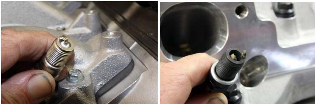
**Left) There's nothing wrong with a standard copper core spark plug, and some power-adder tuners prefer these plugs for helping tune. These plugs are inexpensive and should be considered a consumable. This is an Autolite race plug that is also configured with a side gap. (Right) This melted plug was destroyed when the nitrous system went lean. While it is a**
