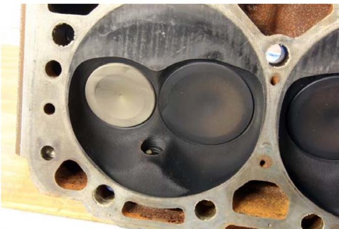
**A spark plug's reach is defined as the length of the threads. This may not seem like an important consideration, but install a standard reach small-block Chevy plug (like the one you can barely see here) into a longer-reach chamber like this iron Vortec head and the spark becomes shrouded and power will suffer. We've seen a 20 hp loss from incorrectly installed plugs like this on a 500 hp engine**
