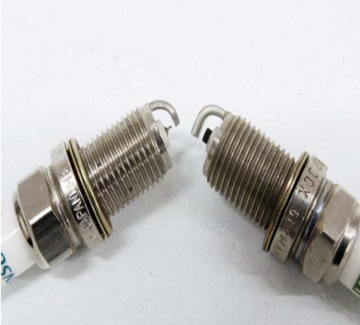
**This compares an extended-nose plug (left) to a standard-reach plug (right). Note how much longer the extended-reach plug's ground strap is compared to the standard-reach. For street engines, the extended-nose is good for part-throttle efficiency. The short-reach is far better for high output engines where the longer ground strap could get hot enough to cause pre-ignition.**
