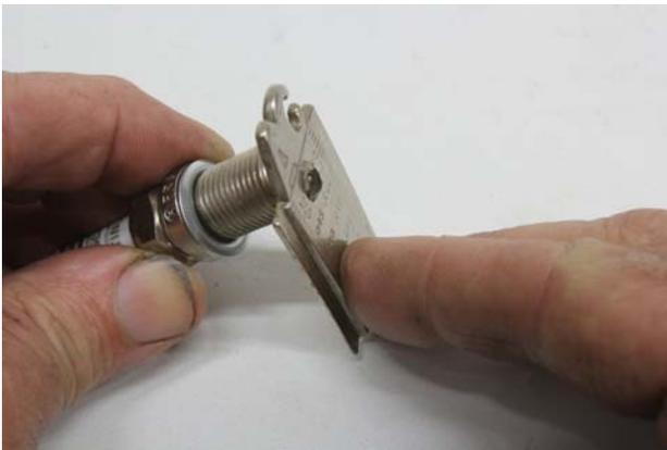
**To increase the plug gap using a simple gap tool, place the end of the ground electrode in the hole and carefully push down on the end of tool. Reeves warns that a too-wide gap can create the situation where the spark fires sideways to the edge of the plug. While the spark still occurs, it can retard the timing by as much as two degrees.**
