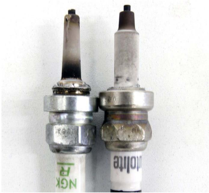
**We removed the threads on these two plugs to illustrate heat range. The plug on the left is a hotter heat range than the plug on the right. Note how the hot plug's ceramic has a longer path from the tip of the plug to where the ceramic contacts the plug's shell and then to the head. The colder plug on the right has a much shorter path for the heat to travel; it pulls heat more efficiently from the plug tip so it will not burn off carbon as easily.**
