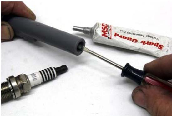
**MSD's Spark Guard is dielectric grease used to protect the boot from sticking to the spark plug and minimize errant spark leakage. Do not smear it on the connector to the spark plug. This grease is an insulator not a conductor. Place a small amount around the inside of the boot. Your ignition system will thank you for your attention to detail.**
