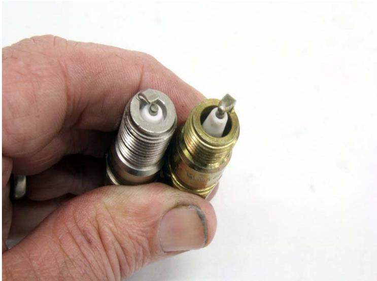
**The addition of precious metal in the center electrode has nothing to do with the heat range of a spark plug. The heat range is designed into the relationship of the ceramic to the plug body. The plug on the left is a cold plug with a shallow ceramic depth. The plug on the right is a much hotter plug with the ceramic connecting with the outer shell much deeper.**
